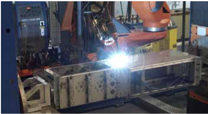
Photo 1: Driescher-Wegberg uses the CLOOS robot system to weld housings of switching systems.
