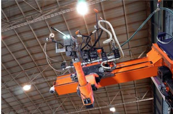
The robot system is equipped with a tactile and an arc sensor which balance the tolerances between the programmed paths and the real component positions.
