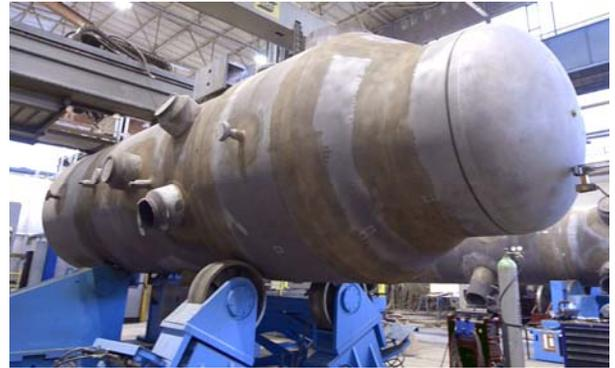
Borsig's custom heat exchangers facilitate efficient cooling of process gases and are used in numerous chemical and petrochemical systems.
