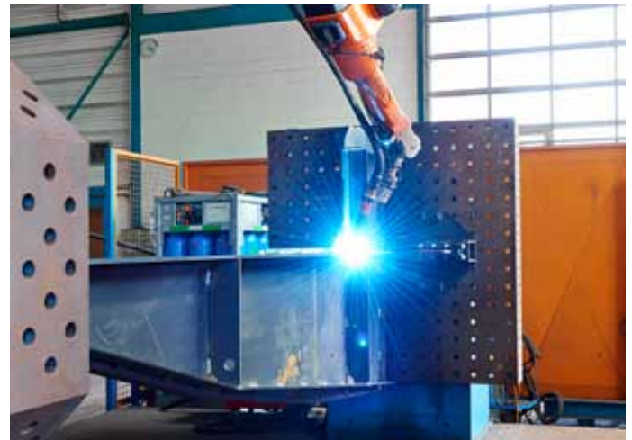
Photo 4: The reach of the 7-axis robot means that it can be easily guided around corners or into niches.
