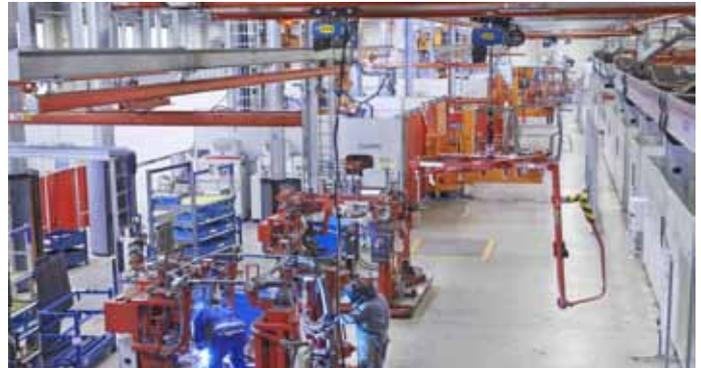
The complex cab-welding production line is more than 70 meters long and comprises a total of twelve stations.
