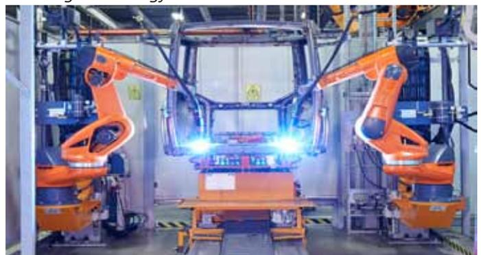
After pre-tacking in the manual stations, the 7-axis robots weld the cabs in automated systems.
