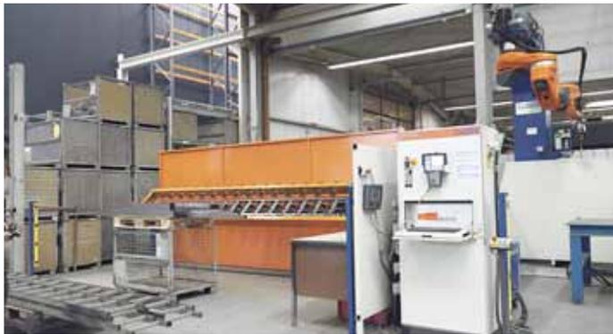
Photo 1: The robot system produces a wide range of different types of ladders for underground engineering.
