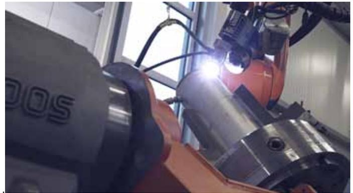
Photo 6: In the past, it took 25 minutes to weld the tank containers manually, now the robot only needs 12 minutes to weld the same component.
