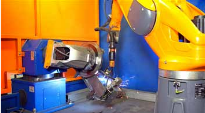
Photo 4: The workpiece positioner consistently brings the component into the optimum welding position.
