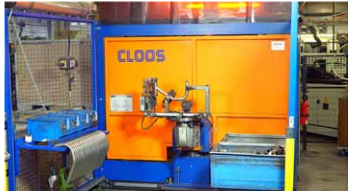
Photo 2: Because of the two-station design, the machine can be charged alternately – an enormous saving in time for the process run.
