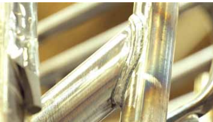
Photo 5: The vehicles must have perfect weld seam in order to fulfill the high safety standards.
